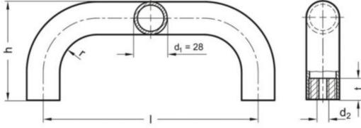
$\begin{array}{ll} d1 &= 20 \\ d2 &= M8 \\ h &= 68 \\ I &= 250 \\ r &= 22 \\ t \min = 15 \end{array}$
